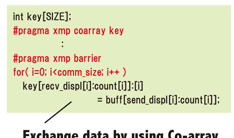
Exchange data by using Co-array
